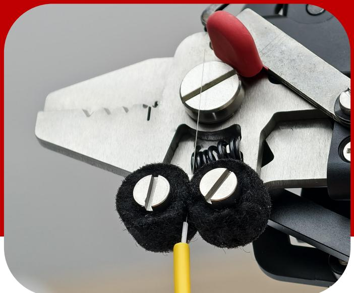
Wipe off the cladding of optical fiber
