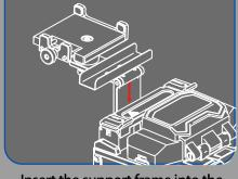
Insert the support frame into the socket of the base, adjust it to a proper height, and tighten the screws
