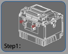
Fasten the fixing base to the back of the splicer with screws
