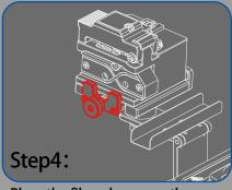
Place the fiber cleaver on the operating table, adjust the depth of the screw to make the rubber pad and the cleaver completely fit
