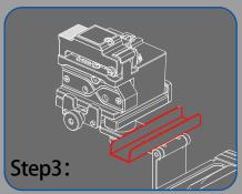
Place the cooling tray on the support frame, and make its hole position coincide with the point position on the support plate
